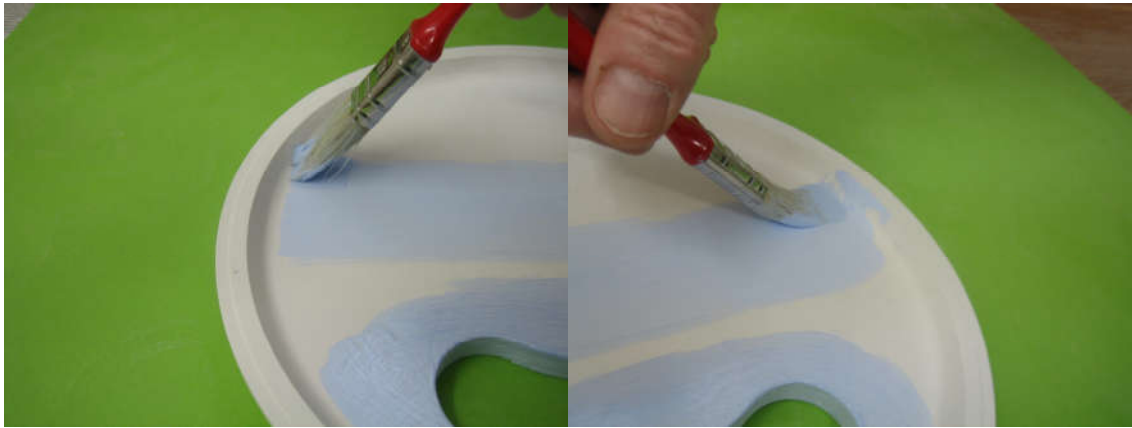
Application by brushing of ALU-STOP LC25 on a transition plate.
